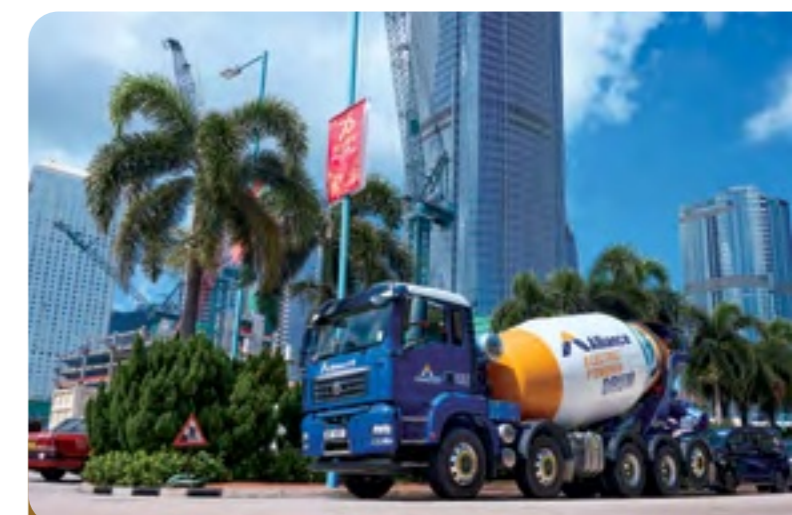
Alliance introduced a battery-electric mixer drum which is fitted onto a diesel truck chassis, achieving up to a 30% reduction in fuel consumption compared with conventional diesel mixer trucks.
